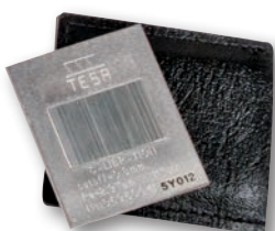
Roughness specimen Ra = 2.97 µm (117 µin)
