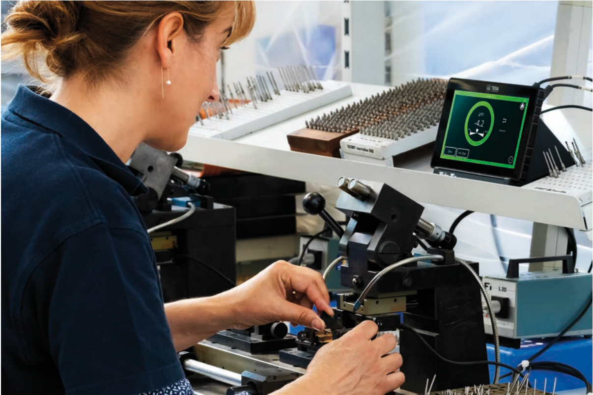
Concentricity measurement before assembly of cylindrical parts
