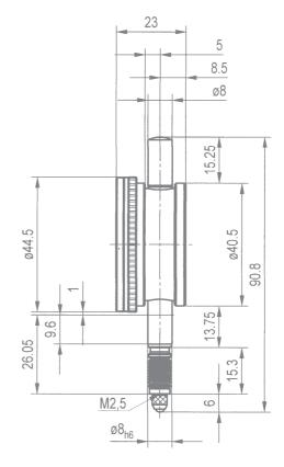
The above dimensioned drawing also applies to the Safety Dial Gauge SI-45 W.
