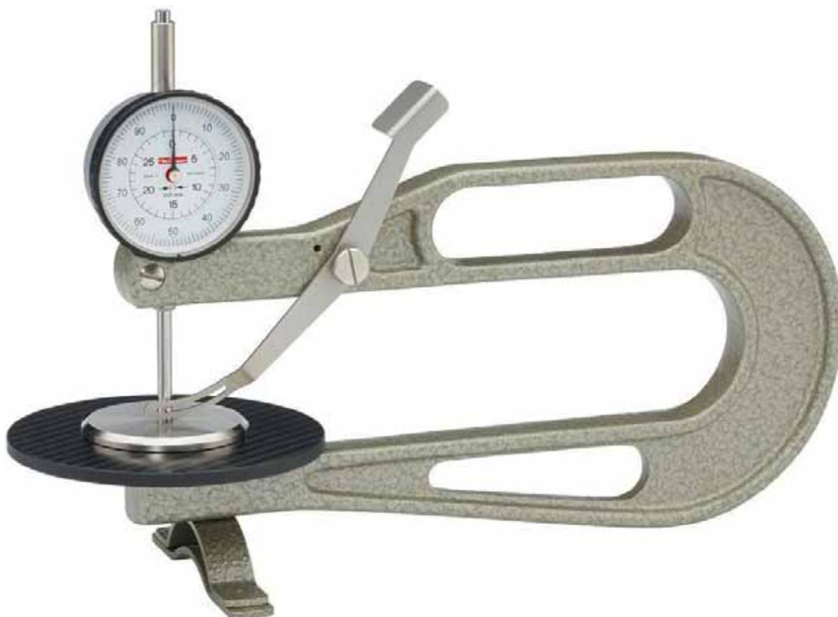
In addition Fleece Dial Thickness Gauge to DIN EN ISO 5084 – edition 1996 can also be supplied. The technical data is the same as above, but it has an upper contact point diameter of 50 mm and a lower contact point diameter of 108 mm. This Thickness Gauge is supplied with an additional weight of 185 gram, which has to be mounted at its top in order to achieve the stipulated measuring pressure. Please request a quotation.
